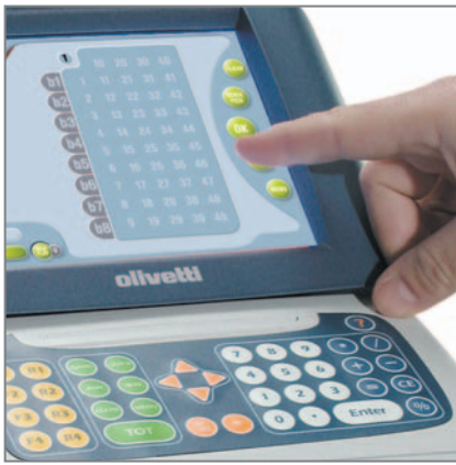
TOUCH SCREEN DISPLAY and integrated keyboard for WEB-oriented services
